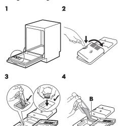
Put the detergent or the multi-tablet in compartment (**A**). If the programme has a prewash phase, put a small quantity of detergent in compartment (B).
